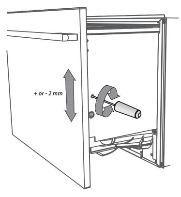
With the front panels fitted, insert an appropriately sized Philips screwdriver into the hole above the door pin and rotate the panels up or down to align the gaps in your cabinetry.
